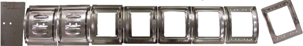
PART DESIGNATION: WASHING MACHINE FRAME DIE DIMENSIONS: 2700*1110 MATERIAL: STAINLESS STEEL 0.5mm DICK
