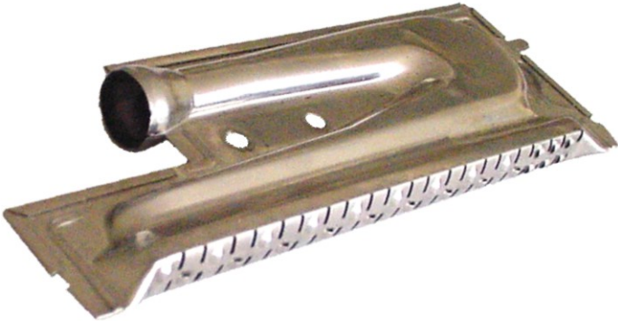
STAMPING FACTORY: TAPEM PART DESIGNATION: WATER HEATER GAS BURNER MATERIAL: STAINLESS STEEL 0.3mm DICK DIE DIMENSIONS: 2100*820 (see die in front page) CADENCE: 50 PARTS/MIN PRODUCTION: WE HAVE ALREADY MADE MORE THAN 120 MILLION PARTS.
